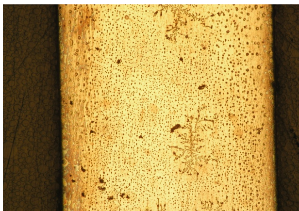
Figure 5. Intercrystalline corrosion, ext. 50x
