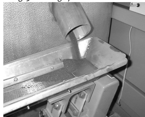
Fig.5. Returning of sifted abrasive
