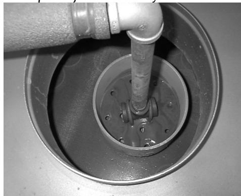
Fig. 3. Cleaning of abrasive material
