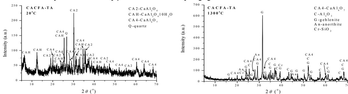
Figure 2. XRD diffractograms of CFA at temperatures 20 and 1300 °C
