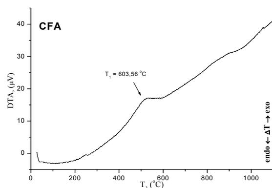
Figure 1. DTA curve of the CFA composite
