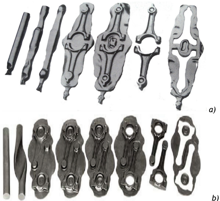
Figure 4. Two-at-a-time conrod forging Error! Reference source not found.
