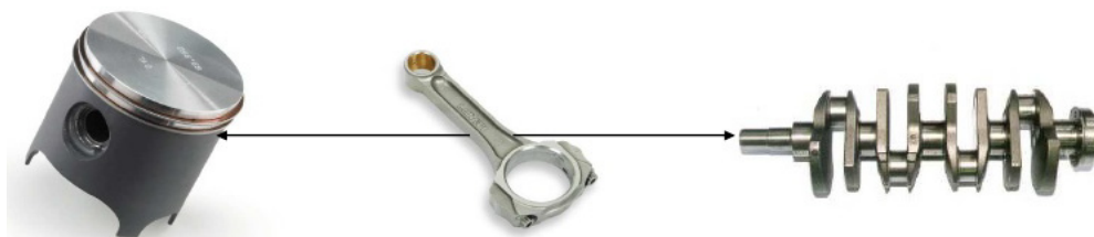
Figure 1. Connection rod converts linear motion of the piston to rotary motion of the crankshaft
