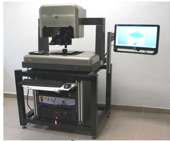
Figure 1. AltiSurf®520 3D surface roughness measuring system
