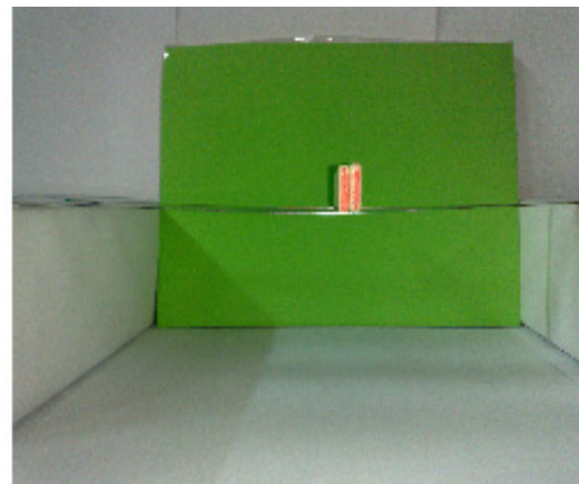
Figure 2. Horizontal Steel Rulers Simulating Supporting Girders
