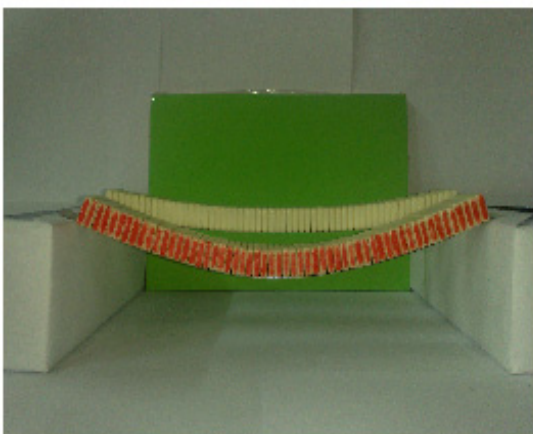
Figure 4. Deflection increase with each Loading increment Central deflections for both rulers were listed in Table1 for each additional two prisms.
