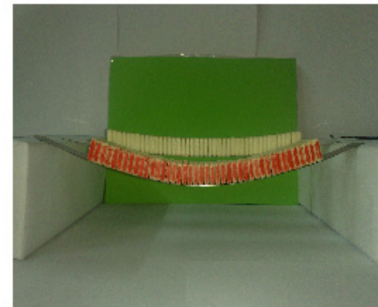
Figure 3. Gluing Plastic Prisms to the Rear Ruler RA
