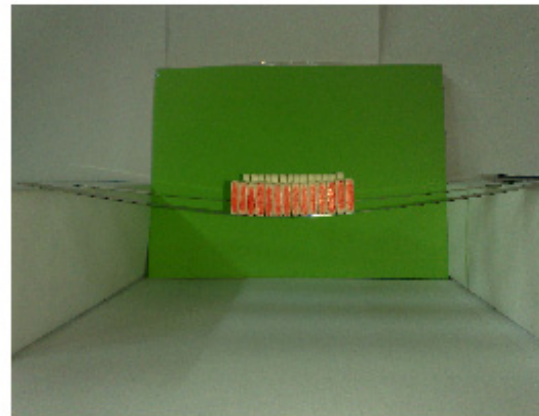
Figure 3. Gluing Plastic Prisms to the Rear Ruler RA
