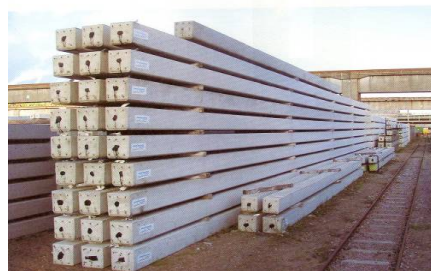
Figure 4. Foundation piles SCC
