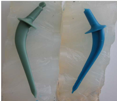
Figure 14. Models of lost wax and silicon rubber mould [5]
