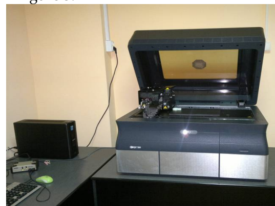
Figure 4. Objet 3D Printer Multifunctional Desktop 30 (Courtesy of Center for Numerical Simulation and Digital/Rapid Prototyping, University "Eftimie Murgu" Resita, Romania)
