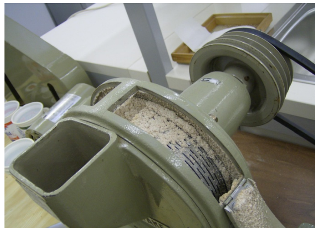
Figure 2. The perforated plate of SATAKE laboratory machines after the debranning
