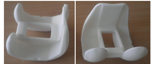
Figure 2. The SLS knee implant geometry
