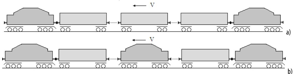
**Figure 1.** The model of the train: a) train with a traction locomotive and the push locomotive, b) train with a traction locomotive and two push locomotives
