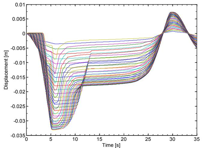
Figure 5. The relative displacements between wagons.
