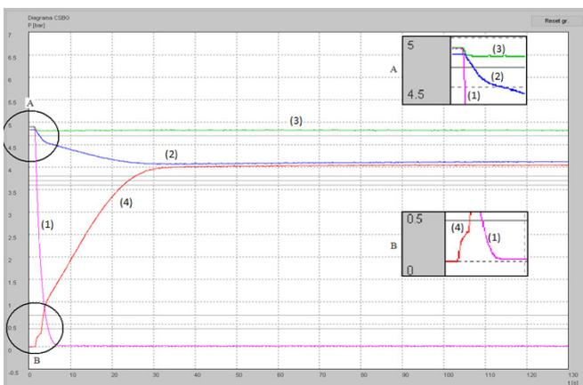
**Figure 2.** The pressure in the braking devices (emergency braking): (1) in the main pipeline; (2) in the auxiliary reservoir; (3) in the operating room of the air distributor; (4) in the braking cylinder [16].
