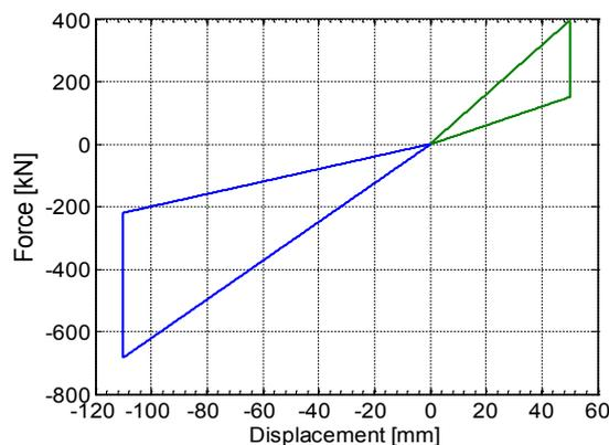
Figure 4. The force-stroke characteristic diagram for the traction, collision and coupling RINGFEDER type device fitting the passenger trains
