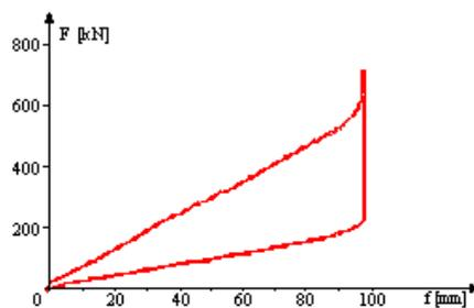
Figure 3. The characteristic of the Ringfeder-type buffer used on freight trains, [10].
