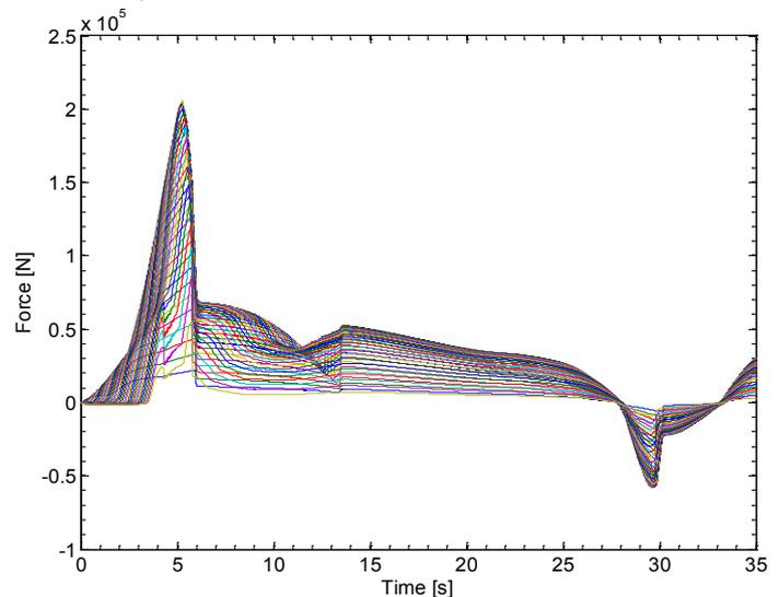
Figure 6. The longitudinal forces between wagons
