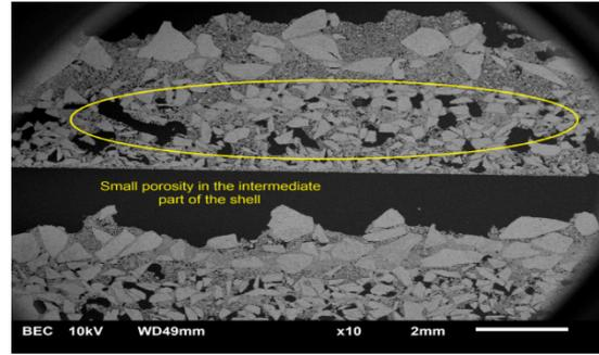
**Figure 5:** SEM picture of newly developed ceramic shell
