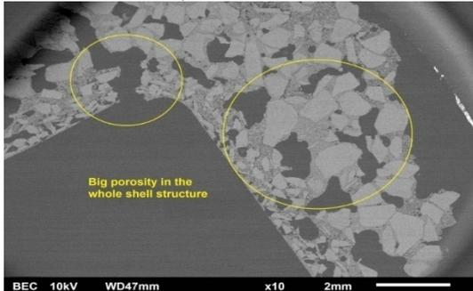
**Figure 6:** SEM picture of a full Molochite ceramic shell
