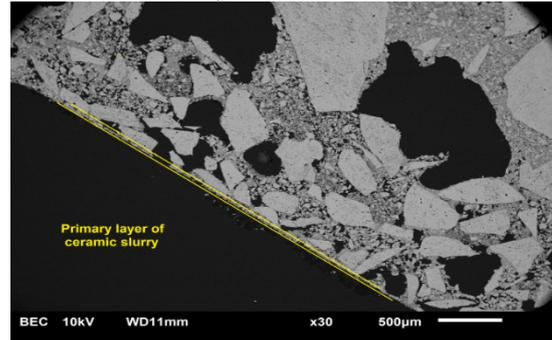
**Figure 7:** Detail of the full Molochite ceramic shell
