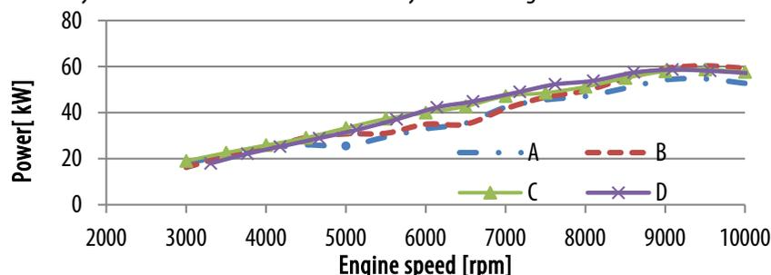
**Figure 11.** Comparison of power characteristics of simulations and measurement
