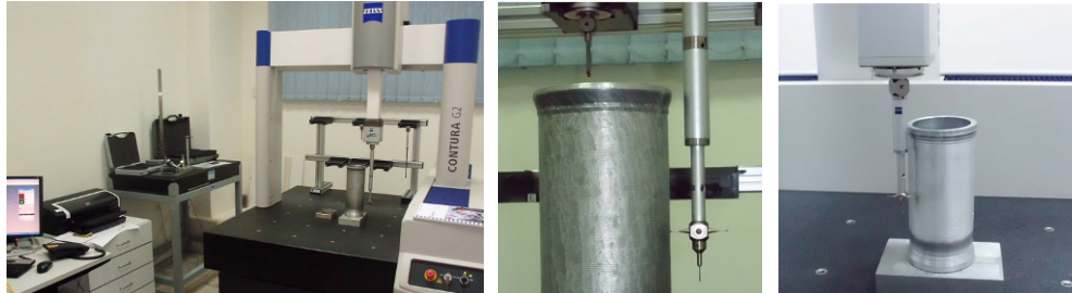
Figure 3. 3D coordinate measuring machine, method of measuring with measuring probe for control of roundness
