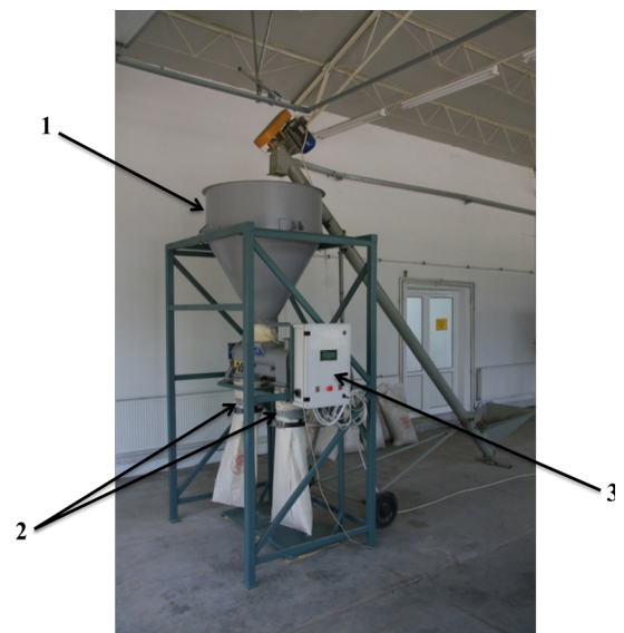
FIGURE 1 – Equipment for weighing and automated management – EWAM - Overview 1 - hopper; 2 – work station1, 2; 3 – automation system
