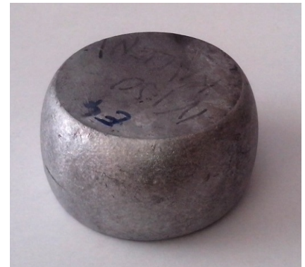
Figure 6. Squeeze casted billet after cooling to the room temperature
