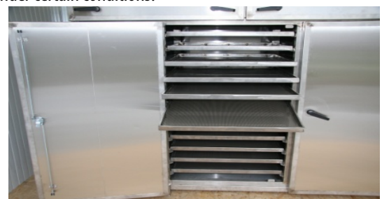
Figure 10 - Dehydrating chamber for fruits and vegetables (Photograph courtesy of Blue Spark Systems)
