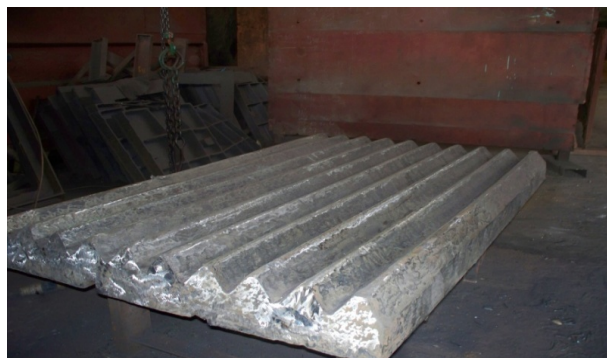
Figure 1. A Locally Produced 500kgamns Jaw Plate in the Factory
