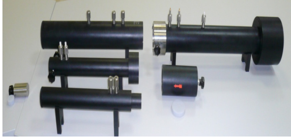
Figure 2. The impedance tube [5]
