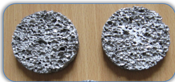
Figure 8. Aluminum foam samples
