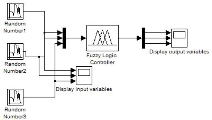
**Figure 9.** Implementation in Matlab-Simulink of the fuzzy system
