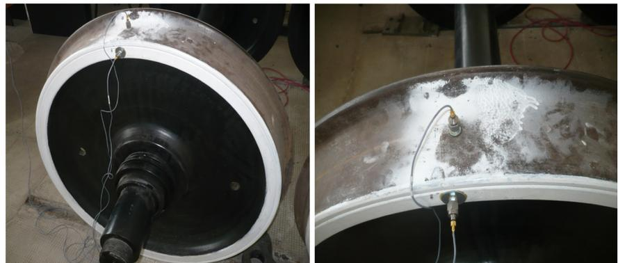
Figure 12. Accelerometers on the rolling surface and lateral surface of the wheel tread.
