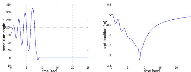
Figure 4. Swing up and stabilization of cart pendulum system
