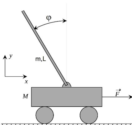
Figure 1. Cart pendulum system
