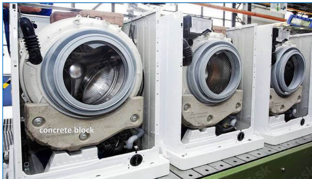
Figure 2. Concrete block inside washing machine (Whirlpool Slovakia)
