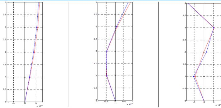
Figure 2. Mode shapes of 20 story-blue and condensed 4 story-red structure
