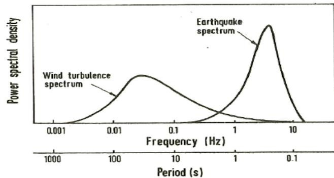
**Figure 1.** Spectral densities of winds and earthquakes
