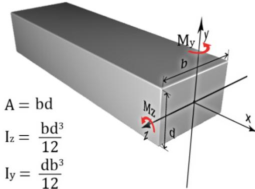
Figure 3. Weak axis of the column  $I_z$
