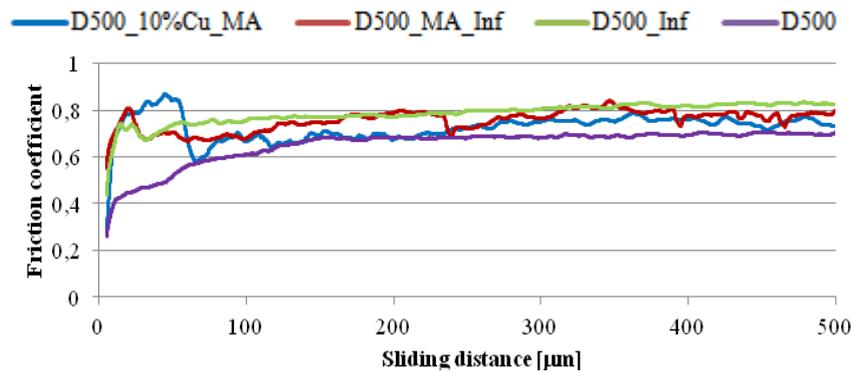
Figure 7: The curves illustrating changes in the friction coefficient as a function of sliding distance for samples pressed at 500MPa compressing pressure – average values
