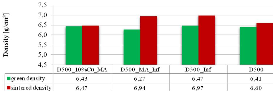
Figure 2: Green and sintered density of investigated samples that were pressed at 500MPa
