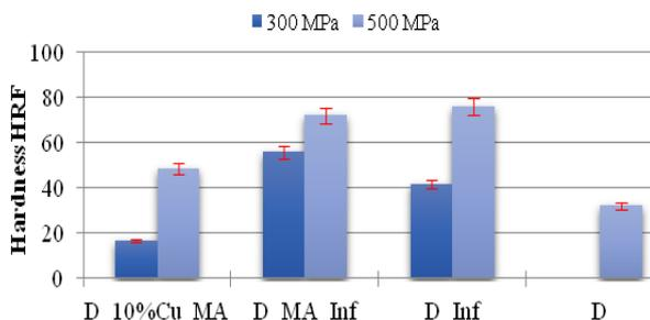
Figure 5: Hardness of investigated samples - value for sample D300 is below HRF scale
