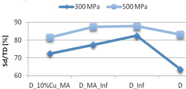
Figure 3: Sintered density to theoretical density ratio for all samples
