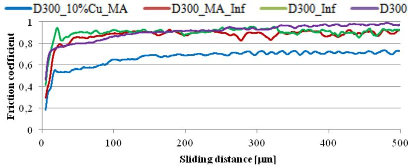
Figure 6: The curves illustrating changes in the friction coefficient as a function of sliding distance for samples pressed at 300MPa compressing pressure – average values
