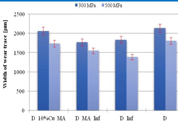
**Figure 9:** Average values of width wear trace for all samples
