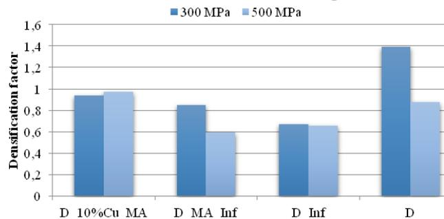
Figure 4: Densification factor for all samples
