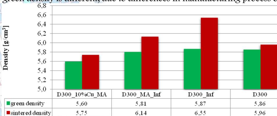
Figure 1: Green and sintered density of investigated samples that were pressed at 300MPa
