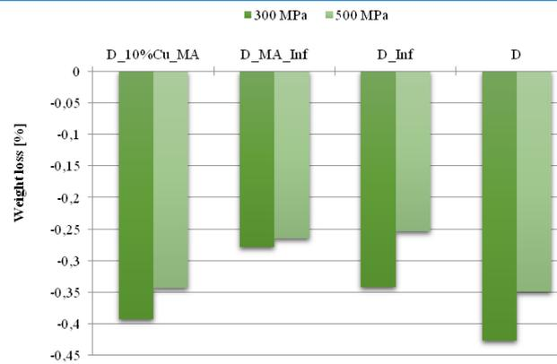
**Figure 10:** Weight loss for all samples
