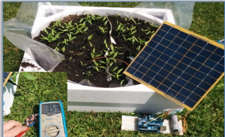
Figure 3. Testing of sensor node for soil-humidity monitoring
