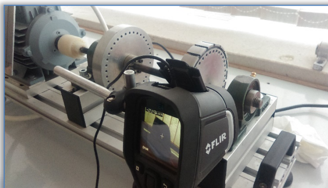
Figure 3 a) FLIR camera, b) temperature measuring
