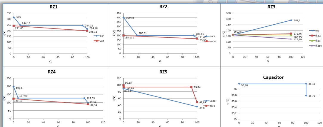
Figure 3. Q-t diagrams for RZ1, RZ2, RZ3, RZ4, RZ5 and condenser
