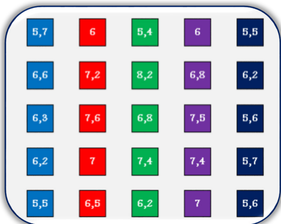
Figure 15. Arrangement of points for the ferrite content measured in the cross sections of sample 7
