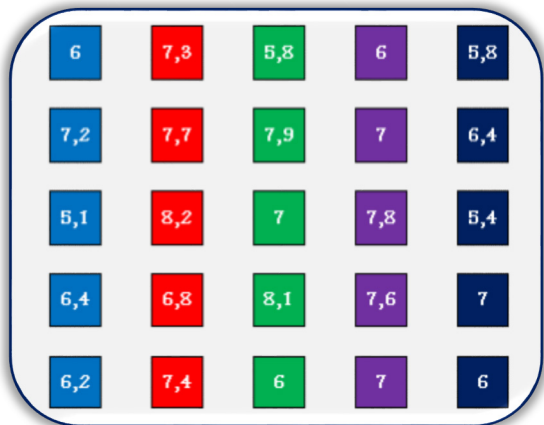
Figure 5. Arrangement of points for the ferrite content measured in the cross sections of sample 2
