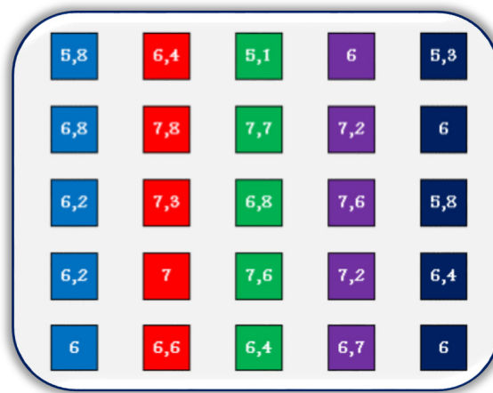
Figure 11. Arrangement of points for the ferrite content measured in the cross sections of sample 5
