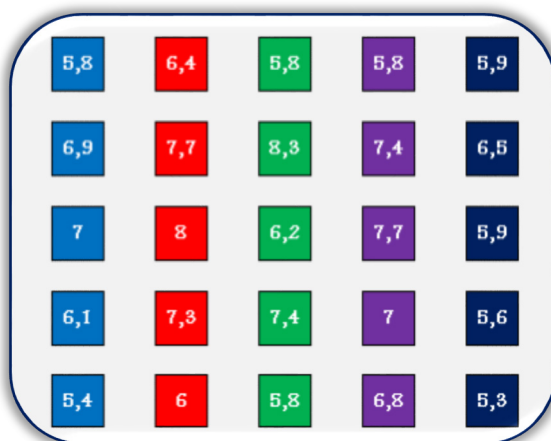
Figure 17. Arrangement of points for the ferrite content measured in the cross sections of sample 8
