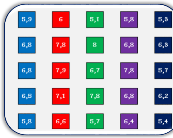
Figure 13. Arrangement of points for the ferrite content measured in the cross sections of sample 6
