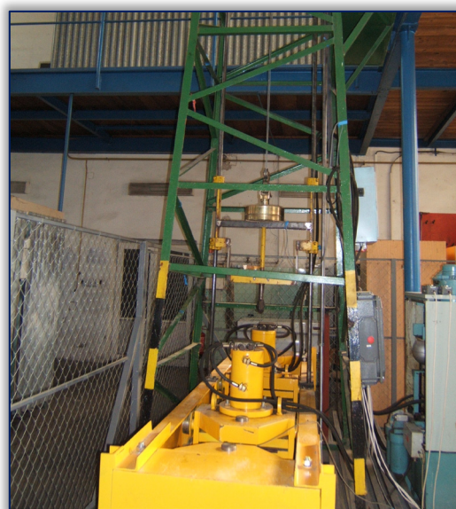
Figure 1. The test device with the drop hammer and impactor details
