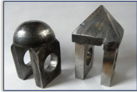
Figure 2. The applied impactor shapes according to the degree of damage. In the case of significant damage, the test was repeated.
