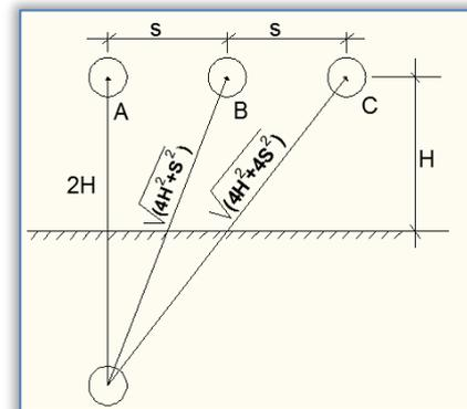
Figure 4. Three-phase horizontal configuration of an overhead transmission line
