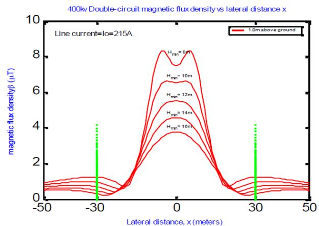
Figure 2. Discuss magnetic field around single & double circuits 400kV transmission line, 1m above ground,  $I_0=1000$
