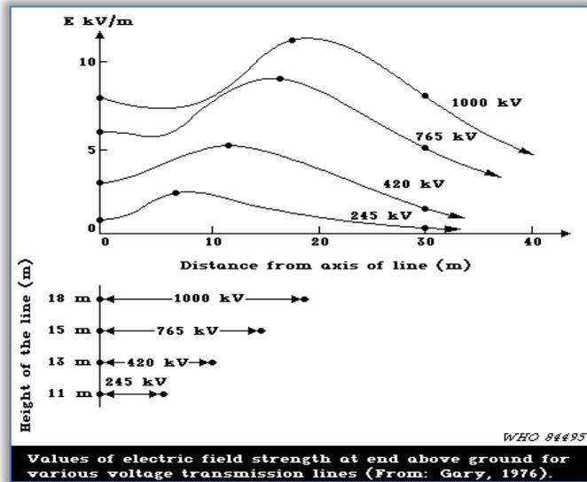
Figure 1. Illustrates the electric fields of several transmission lines
