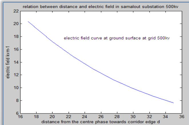
Figure 5. Relation curve between the distances coordinates with the electric field
