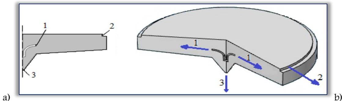
Figure 2. Secondary clarifier scheme:
