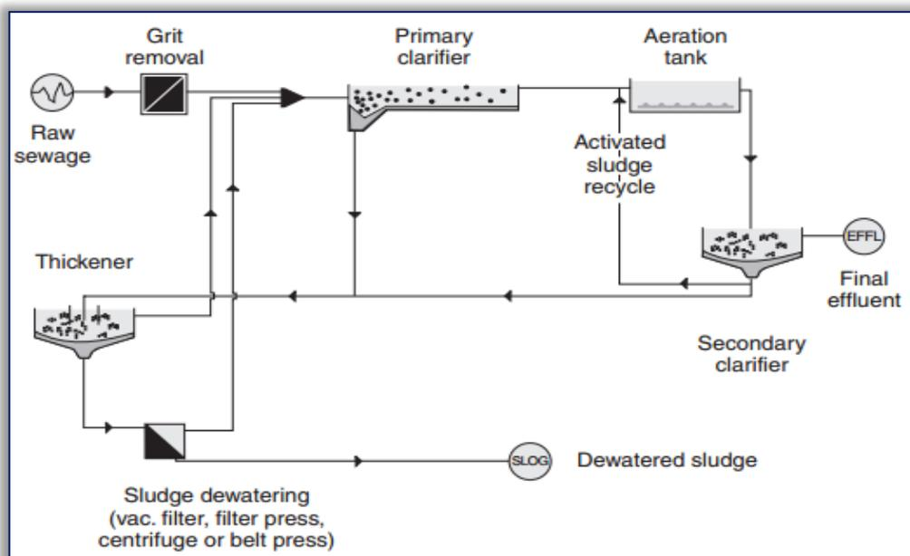
Figure 1. Schematic representation of a wastewater treatment plant equipment [4].
