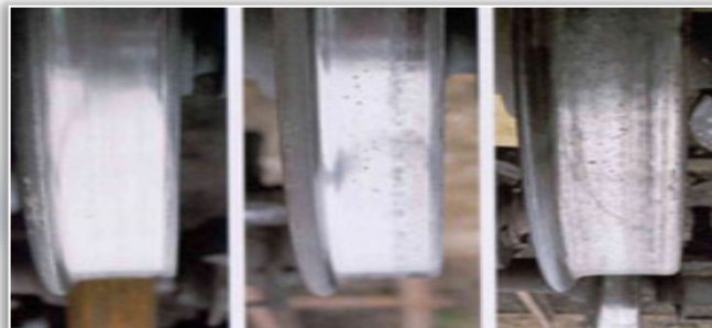
Figure 1. Several grades of wear on the wheel
