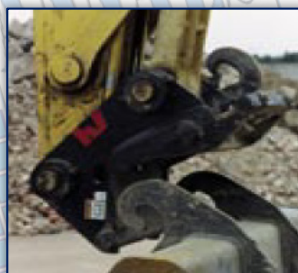
Figure 10. Different positions of the hydraulically operated quick coupling with mobile fork from Verachttert [7]
