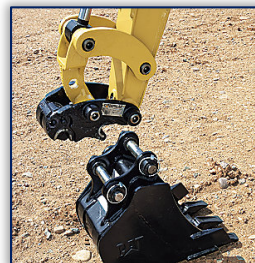
Figure 3. Quick coupling system, designed by the TEFRA Company [2]
