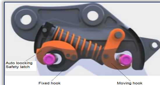
Figure 4. Detail of the mechanical coupling system from Figure 2 [2]
