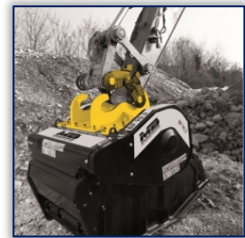
Figure 7. Articulated mechanical quick coupling designed by the company MB Spa [5]
