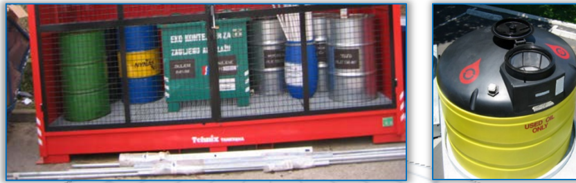
Figure 2: Storage of oily waste [3] and containers for oil safe disposal
