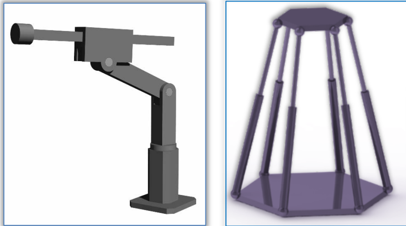
Figure 1 – Serial structure versus parallel structure robot type
