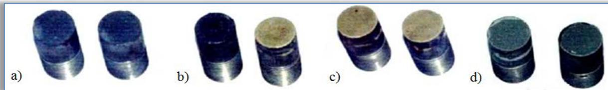
Figure 1. Undesirable possible fracture locations: a) through the bond coating, b) at the bond coating / ceramic coating interface c) through the ceramic coating and d) at the ceramic coating / glue interface [3].
