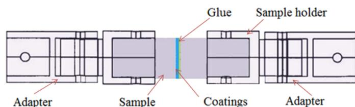
Figure 2. Schematic representation of the adhesive tensile test
