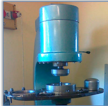
Figure 2. Deep drawing machine with tools
