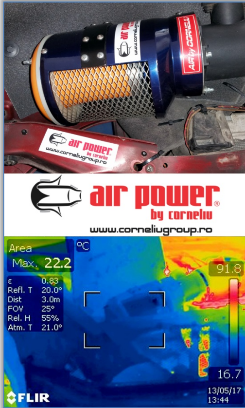
Figure 6. The thermal field in the air filter area captured with a thermographic camera; a.(alternative1);b. (alternative 2)
