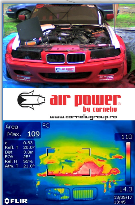
Figure 5. The thermal field in the engine compartment captures with a thermographic camera; a.(alternative 1); b. (alternative 2)
