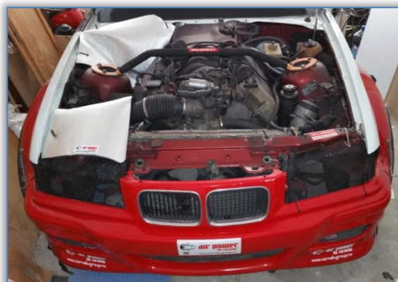
Figure 2. Engine compartment-setting of integrated thermal baffle plate
