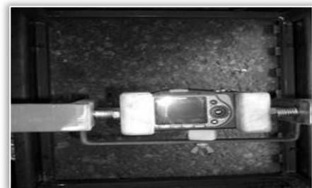
Figure 3 - Digital camera mounted in sealed box on the autonomous robot
