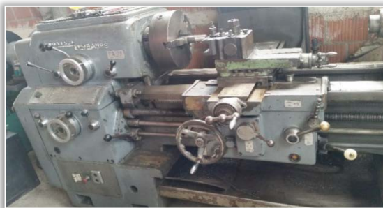
Figure 4. Lathe machine PA22 Figure 5. Measurement microscope Carl Zeiss
