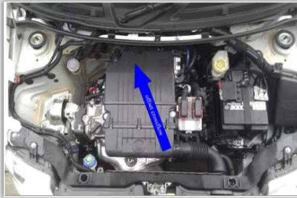
Figure 2. The air circulation through the air filter [3]
