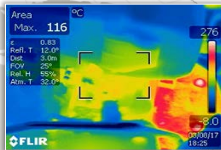
Figure 14. Thermal field in the upper part of the engine
