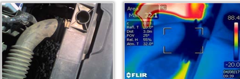
Figure 5. The thermal field on the surface of the connection inlet of the air filter
