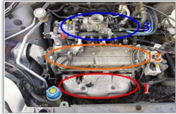
Figure 3. Overview of the engine. 1-exhaust manifold; 2-engine; 3-intake manifold [5]
