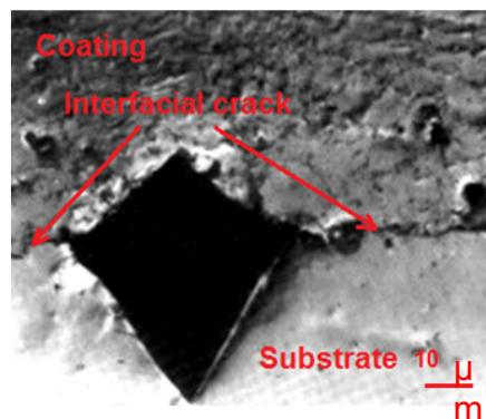
Figure 2. (BM) the geometry of the indentation with the crack at the interface initiated by the critical load
