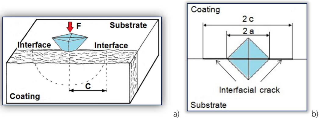
Figure 1. a) A schematic view of an indentation test; b) the geometry of the indentation
