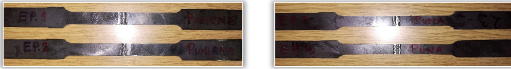
Figure 3. Test tubes prepared for tensile testing
