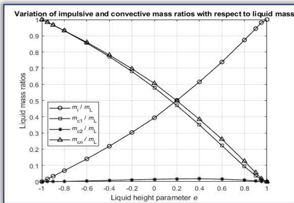
Figure 2: Variation of impulsive and convective mass ratios with respect to total liquid mass
