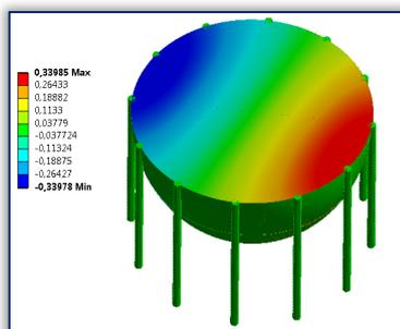
Figure 7: First convective mode of oscillation
