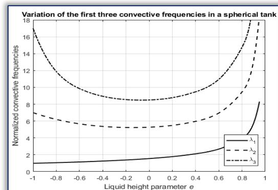
Figure 6: Variation of the first convective frequencies for liquid height parameter  $e$
