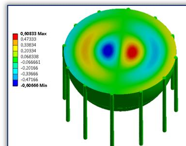
Figure 9: Third convective mode of oscillation
