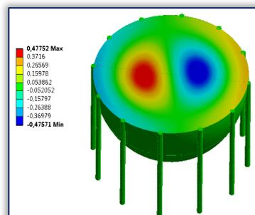
Figure 8: Second convective mode of oscillation
