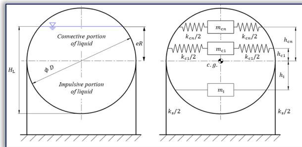
Figure 1: Mechanical model of a spherical tank containing liquid
