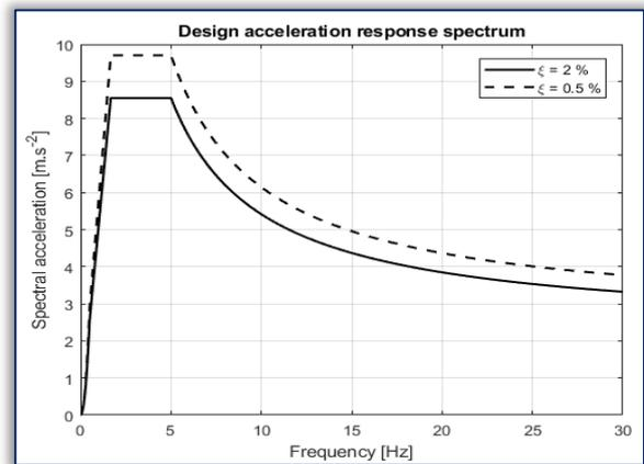
Figure 4: Design acceleration response spectrum according to Eurocode 8
