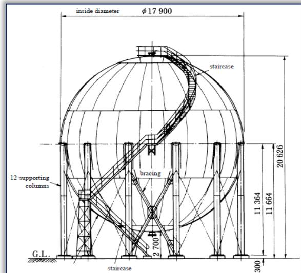
Figure 3: Investigated model of spherical liquid storage tank [14]
