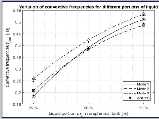
Figure 10: Variation of convective frequencies for different liquid heights
