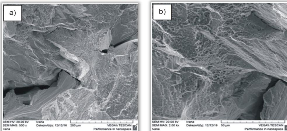
Figure 2. Microfractography of CuAlNi SMA in as-cast state at different magnifications
