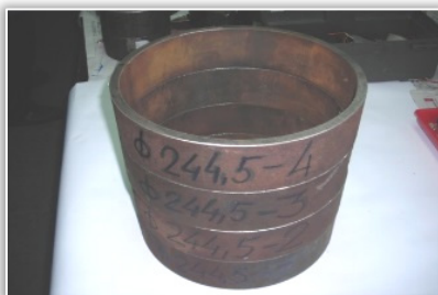
Figure 3a. Saw cut rings samples from pipe products
