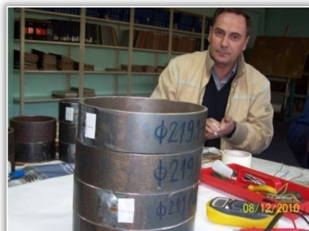
Figure 3c. Location of the strain gage on rings surface
