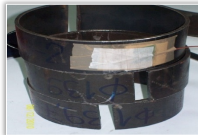
Figure 3b. Slitting pipe rings from one side
