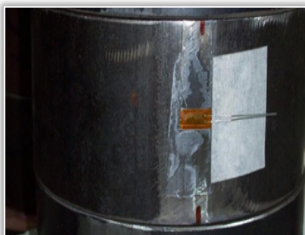
Figure 3c. Location of the strain gage on rings surface
