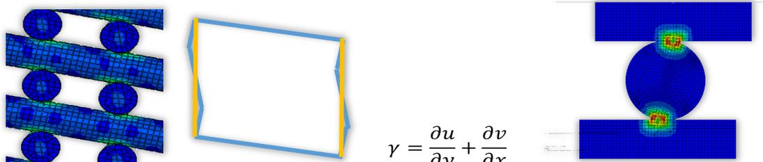
$$\gamma = \frac{\partial u}{\partial y} + \frac{\partial v}{\partial x}$$
