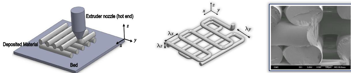
Figure 2. Additive manufacture of porous lattices via a controlled fused deposition modelling process. Schematic diagram of the process (left), control of porosity via lattice spacing (center), SEM micrograph of the manufactured lattice (right).
