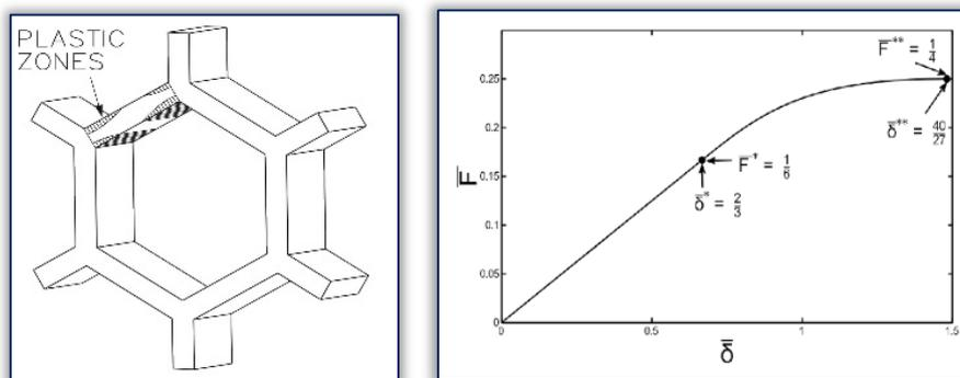
Figure 1. A hexagonal cell from an infinite honeycomb showing details of the plastic zones formed during elasto-plastic deformation of a remotely loaded honeycomb sheet (left), a "master-curve" for response of such lattices (right [4]).
