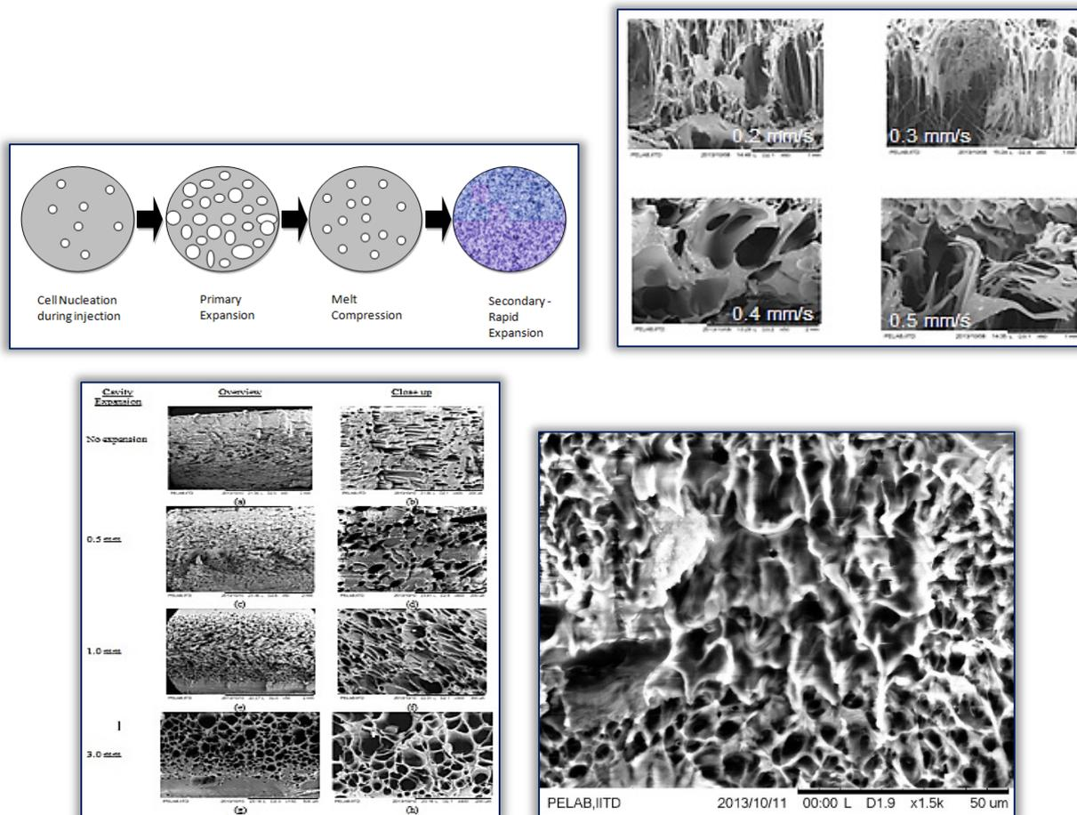
Figure 4. Porous material manufactured via expandable cavity moulding. Schematic of the process (top left), the effect of expansion rate on cell morphology of propylene foam (group of four micrographs, top right), the effect of expansion stroke on cell morphology of PLA foam (group of eight micrographs, bottom right), high-resolution detail (bottom right).
