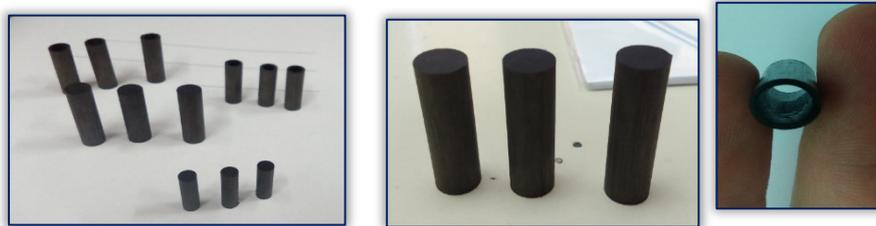
Figure 1. Test specimen prepared for compression testing
