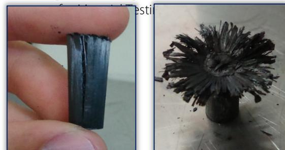
Figure 3. a) The expected crack in case of successful tested specimens under compression; b) The specimen crack tested under compression in case of test results dispersion
