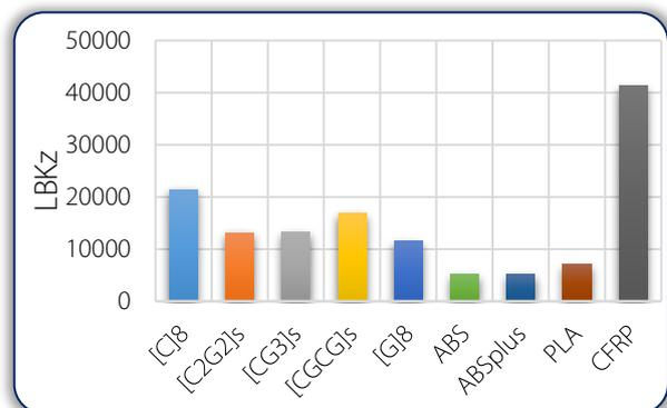
Figure 4. Comparison of LBKz factor values for different materials
