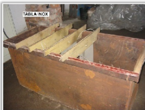
Figure 4. Electrolysis battery with 5 PbSb anodes and 4 stainless steel cathodes with dimensions: 4.5 x 2.8 dm for the Zn extraction from the ZnSO_4 solution
