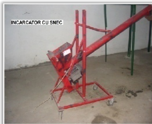
Figure 5. Screw feeder for fractional introduction of brass dross into the acidic solution for solubilization
