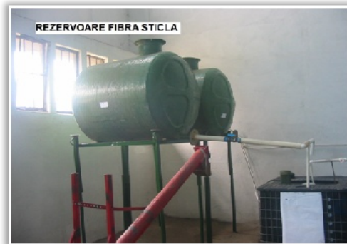
Figure 3. Sulfuric acid tanks and electrolyte waste solution intended for the solubilization of brass dross
