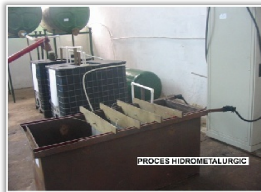
Figure 6. Overview of the brass cross processing section on the solubilization - metal precipitation - electrolysis sequences for the metallic Zn extraction
